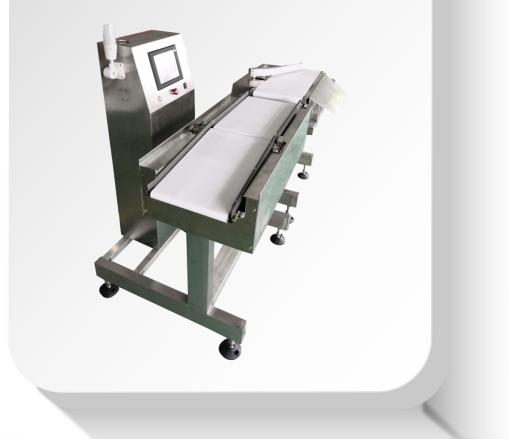
**Principle:** Dynamic online weighing and overweight & underweight rejection.
